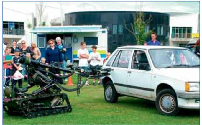
Watched by visitors to Blue Light Day, held this year at the Tidworth Leisure Centre, 721 Sqn EOD RLC demonstrated how the remote-controlled "wheelbarrow" can easily open a car door to search inside a vehicle for a suspect package or explosive device.
